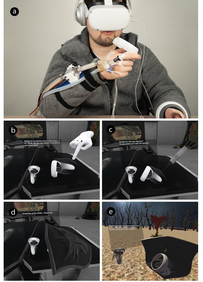
Figure 15: (a) VR user study setup. VR scenes: (b) user experiencing gentle touch, (c) user receiving needle injections, (d) user activating a power shield, and (e) user defending against flower-shaped monster attacks.
